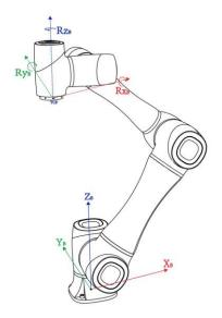
Figure 2.13 Base coordinate system of CR5 robot
