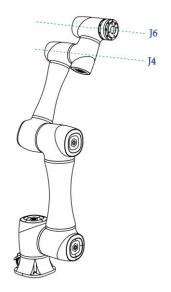
Figure 2.16 Wrist singularity point
