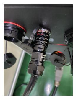
Figure 4.3 Connecting emergency stop switch
