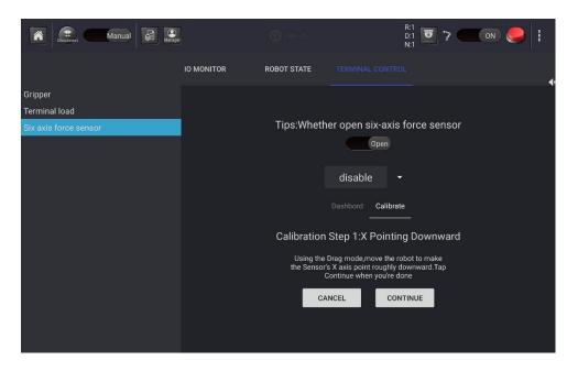
Figure 5.33 Calibrate X-axis
