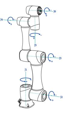
Figure 2.12 Joint coordinate of a CR5 robot
