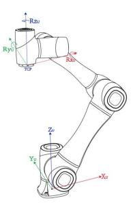
Figure 2.15 The default User coordinate system of CR5 robot
