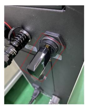
Figure 4.4 Connecting WiFi module
