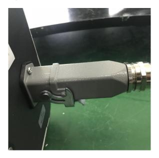
Figure 4.2 Connect controller and robot by heavy-duty cables
