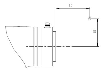
Figure 2.4 End-effector load diagram
