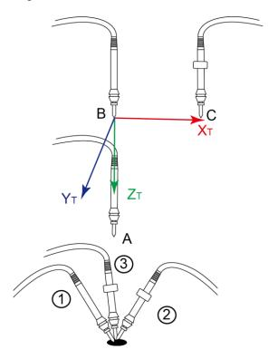
Figure 5.11 Three points calibration method (TCP+ZX)
