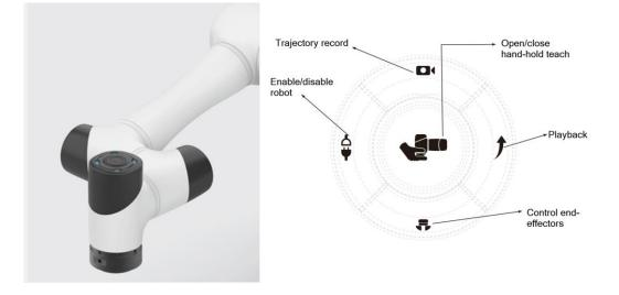
Figure 2.19 Keys on robot
