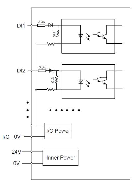
Figure 3.6 Simple digital input circuit
