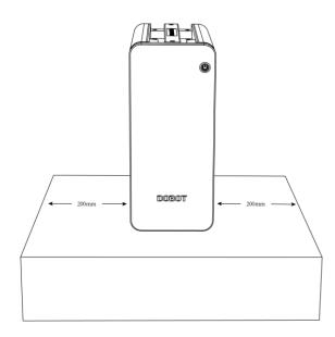
Figure 4.1 Installation space requirement
