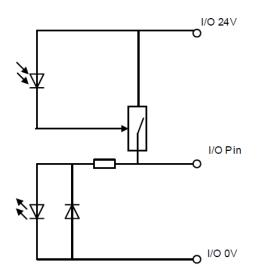
Figure 3.7 Simple digital output circuit
