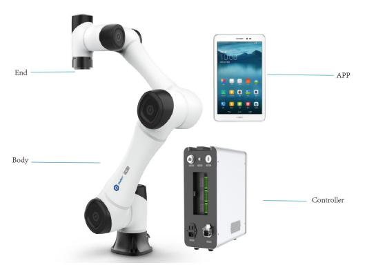
Figure 2.1 Robot system
