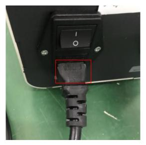
Figure 4.5 Connecting to Power Supply
