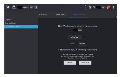
Figure 5.35 Calibrate Y-axis
