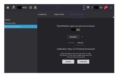
Figure 5.37 Calibrate Z-axis
