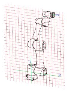
Figure 2.17 Shoulder singularity point
