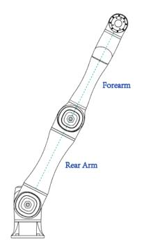
Figure 2.18 Elbow singularity point
